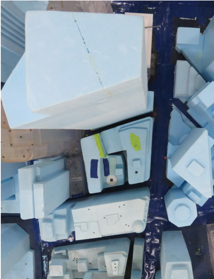
Figure 4: Configuration A existing site model in the wind tunnel viewed from above.
